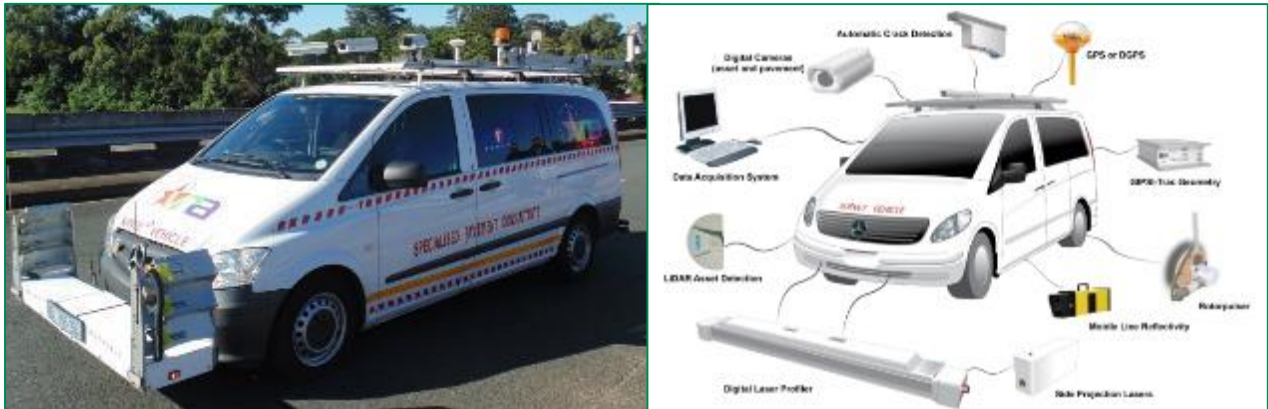
Figure 4 1: The road survey vehicle
